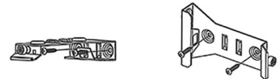
FIGURE 9 Mounting Bracket on a Flat Surface
